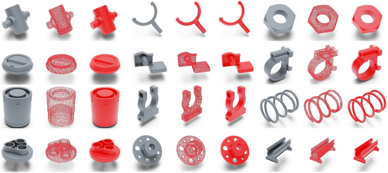
Fig. 10. Results of our method, each set shows the ground truth, the used point clouds, and the rendering of our reconstruction.
